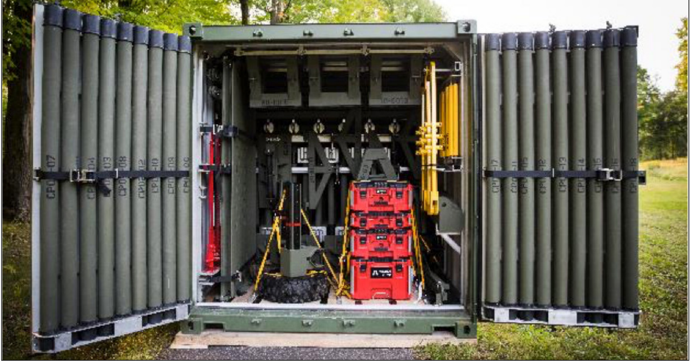
Figure 1. The LVTB is designed to be a Bridge in a Box that can quickly be shipped and deployed for emergency situations.
