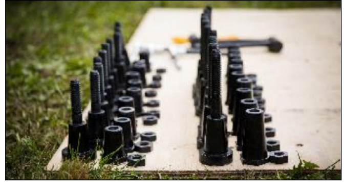
Figure 6. Only 28 bolts are required to assemble the LVTB.
