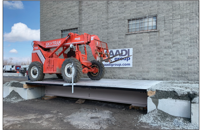
Figure 1. Deflection test of the aluminum bridge deck at MAADI’s facility.
