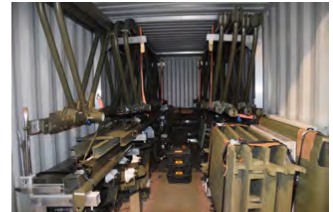
Fig 5.103 Inside a 6.1m container all the components of the prototype bridge
