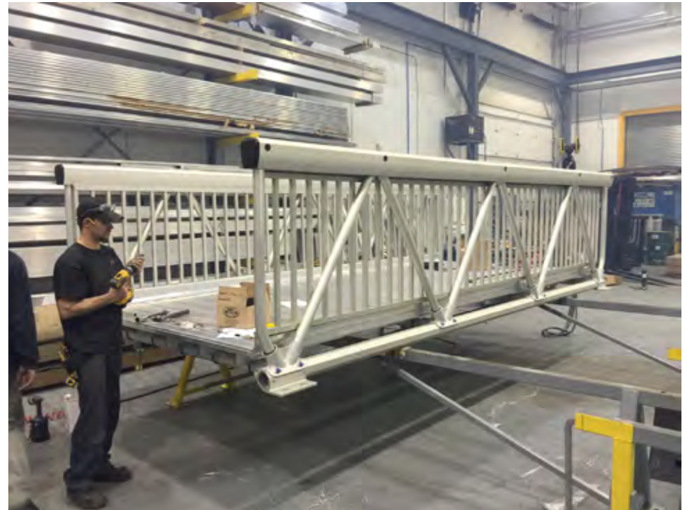
Fig 5.110 A silver anodised Make-A-Bridge ™ pedestrian footbridge at MAADI Groups factory awaiting installation in Calgary, Alberta
