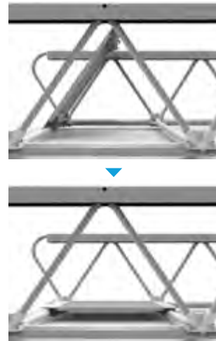
Fig 5.108 Decking assembly of the Deployable Military Bridge
