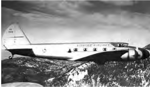
Fig 2.3 The Boeing 247D is regarded as the first 2000 series aluminium alloy semi-monocoque airliner, 1933
