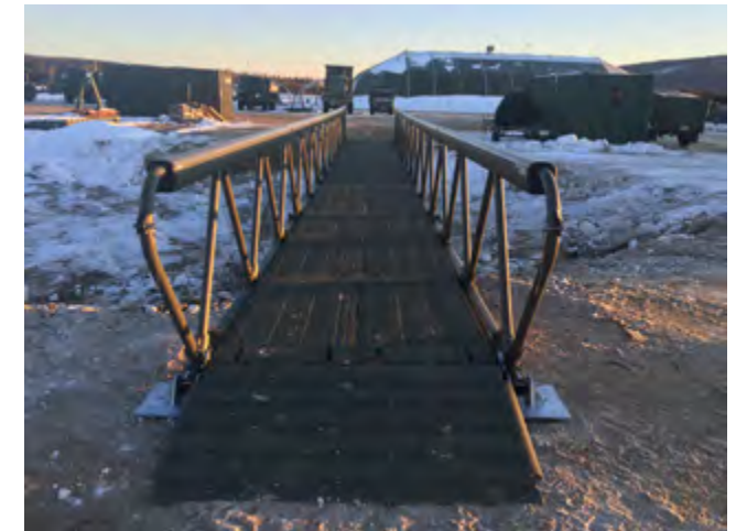
Fig 5.102 Rapidly deployable military bridge on test by the Canadian Army
