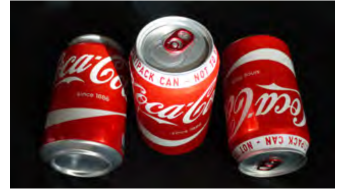
Fig 2.4 An aluminium Coke can, with 3004 aluminium alloy deep drawn body and 5182 alloy cap
