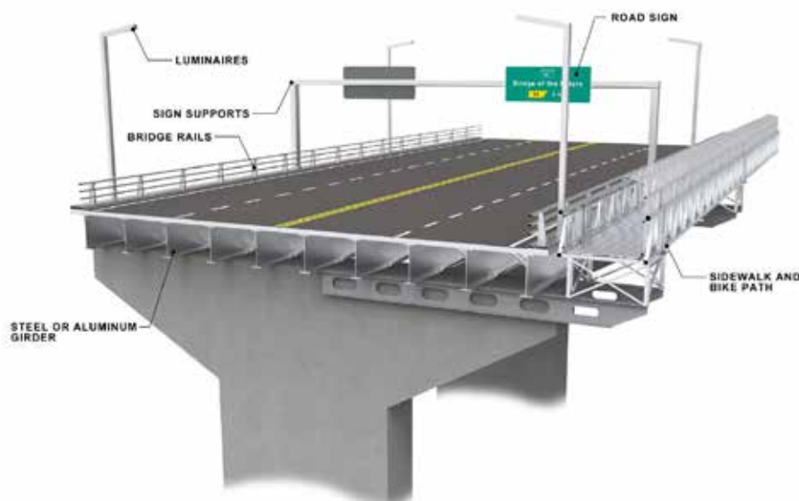
Figure 8. Use of aluminum in secondary bridge components.
